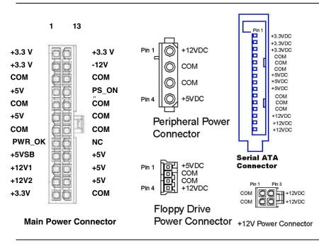
Figure 14. TFX12V Connectors (Pin-side view, not to scale)
